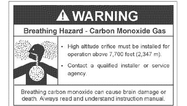
Water heaters covered in this manual have been tested and approved for installation at elevations up to 7,700 feet (2,347 m) above sea level. For installation above 7,700 feet (2,347 m), the water heater's Btu input should be reduced at the rate of 4 percent for each 1,000 feet (305 m) above sea level which requires replacement of the burner orifice in accordance with the National Fuel Gas Code ANSI Z223.1/NFPA 54. Contact your local gas supplier for further information.
